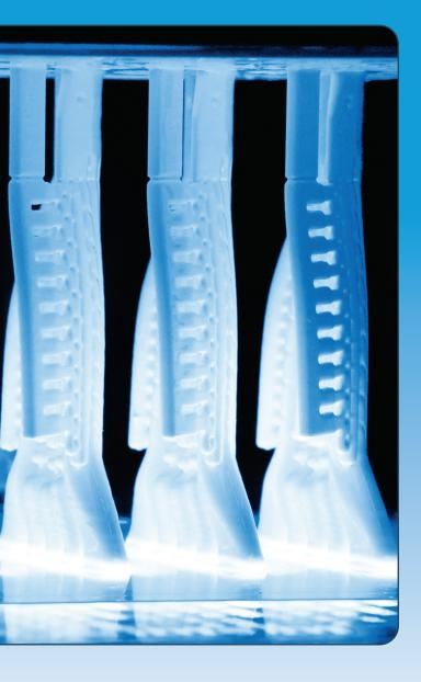
Digital Light Processing, or DLP, is a printing technique known for its ability to print fine features with a high resolution and low surface roughness. It is proving to be effective for 3D printing of shells and cores for investment casting.
