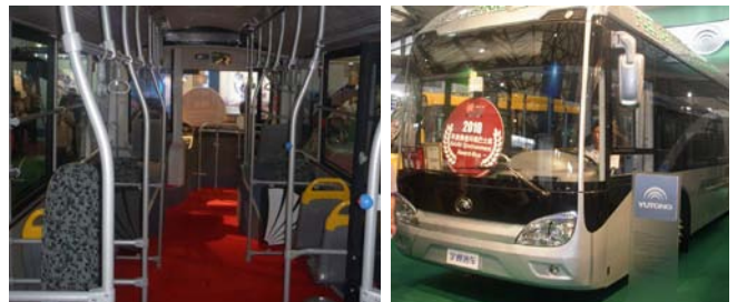
Thousands of magnesium alloy handrails are installed in Chinese Yutong city buses. © Photos courtesy of Beijing Guangling Jinghua Science & Technology Co., Ltd. Used with permission.
