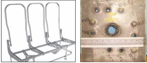
Aircraft seats (left) and armored vehicles (right) plan to use high-strength magnesium alloys, cast using newly-designed DC casting equipment and methodology. © Photos courtesy of Magnesium-Elektron UK. Used with permission.
