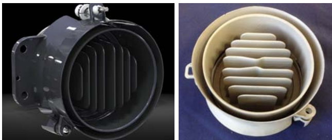
Magnesium combined with investment casting yields a high-powered LED light with integral heat sink, creating high-performance LED automotive lighting. © Photos courtesy of Aristo-Cast, Inc. Used with permission.
