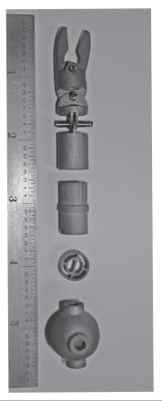
The resulting prototype assembly forms a hand-held light-weight set of forceps made of 316L stainless steel which meets all requirements for durability and surgical instrumentation.
