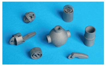
This series of miniature investment castings also features intricate detail and thin walls (0.0460" x 0.825" long at 0.040" wall thickness). The castings are assembled to make handheld articulating laparoscopic forceps to aid in surgery.
