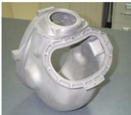
Investment cast diving helmet has cast in features which were previously machined.
