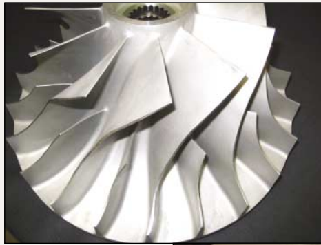
This impeller (above) achieved tight tolerances with good dimensional consistencies after it was cast from a plaster mold (r) through Morris Bean's Antioch process.
