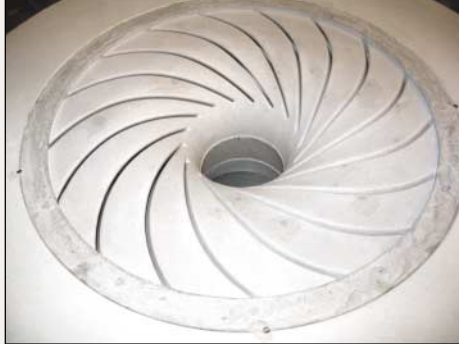
This impeller (above) achieved tight tolerances with good dimensional consistencies after it was cast from a plaster mold (r) through Morris Bean's Antioch process.
