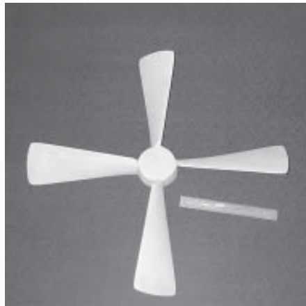
Finished 1913 Jeffery cooling fan (left) and original part (above) from which the new design was made.
