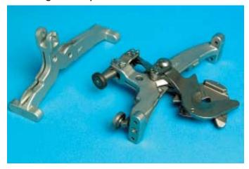
The virtually unlimited choice of alloys in the investment casting process allowed the conversion of a die cast cross arm used in food processing from aluminum to stainless steel for improved performance.
